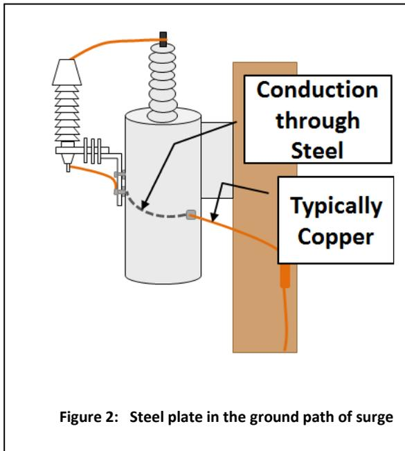
Figure 2: Steel plate in the ground path of surge
